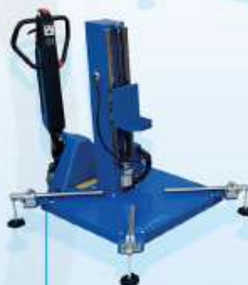
CSM002-2WD: TROLLEY WITH ADJUSTABLE LIFTING COLUMN. Electric motorized trolley. Column H= 1060 mm and stroke 600mm. Handling through brushless motor 400W – 220 V. Piloting by electronic accelerator and up and down buttons. Total weight 480 kg (1058 lb).
