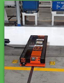
Volkswagen AG/Body 10. 2000 operating since Apr'10 operating since Apr'10 Hydraulic lifting Accurate movements in narrow area
