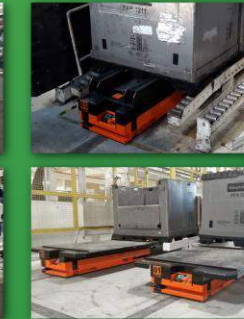
Fitradia/PSA - 2000/Body assembly 5. 2000 operating since Nov'10 operating since Nov'10 Hydraulic lifting Accurate movements in narrow area
