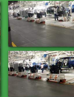
Volkswagen AG/Body assembly 16. 2000 operating since Apr'10 operating since Apr'10 Automatic pin Accurate movements in narrow area
