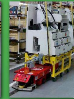
PSA/PSA Group 4. 2000 operating since Nov'10 Automatic battery charging Interaction with existing infrastructure 3 off 300m circuits
