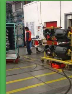
PSA/Volkswagen Hexabot 7. 2000 operating since Apr'10 operating since Apr'10 Hydraulic lifting Wireless communications and management
