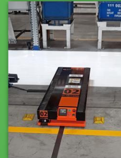
Volkswagen AG/Tronby 10 sqm operating circuit 24/7 Hydraulic lifting Accurate movements in narrow area
