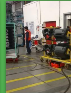
PSA/Volkswagen AG/Tronby 2. 10 sqm operating circuit 24/7 Hydraulic lifting Wireless communications and management
