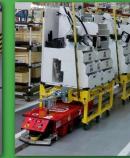
PSA/PSA Group 4. 2000 sqm operating circuit 24/7 Automatic battery charging Interaction with existing infrastructure 3 off 300m circuits
