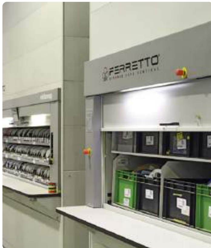
Rotating storage systems for integrated circuit components
