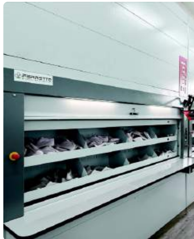
Rotating storage systems for manufacturing facilities (footwear industry)
